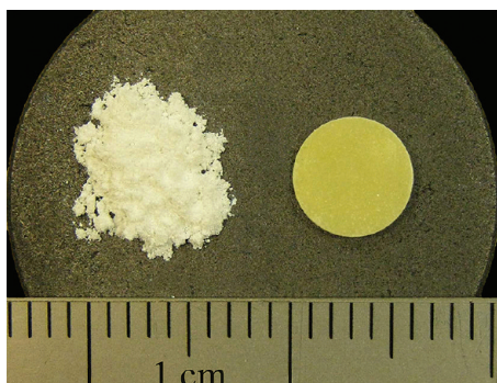
Figure 6. Phase-pure \text{Bi}_2\text{Ti}_2\text{O}_7 powder and pellet.
